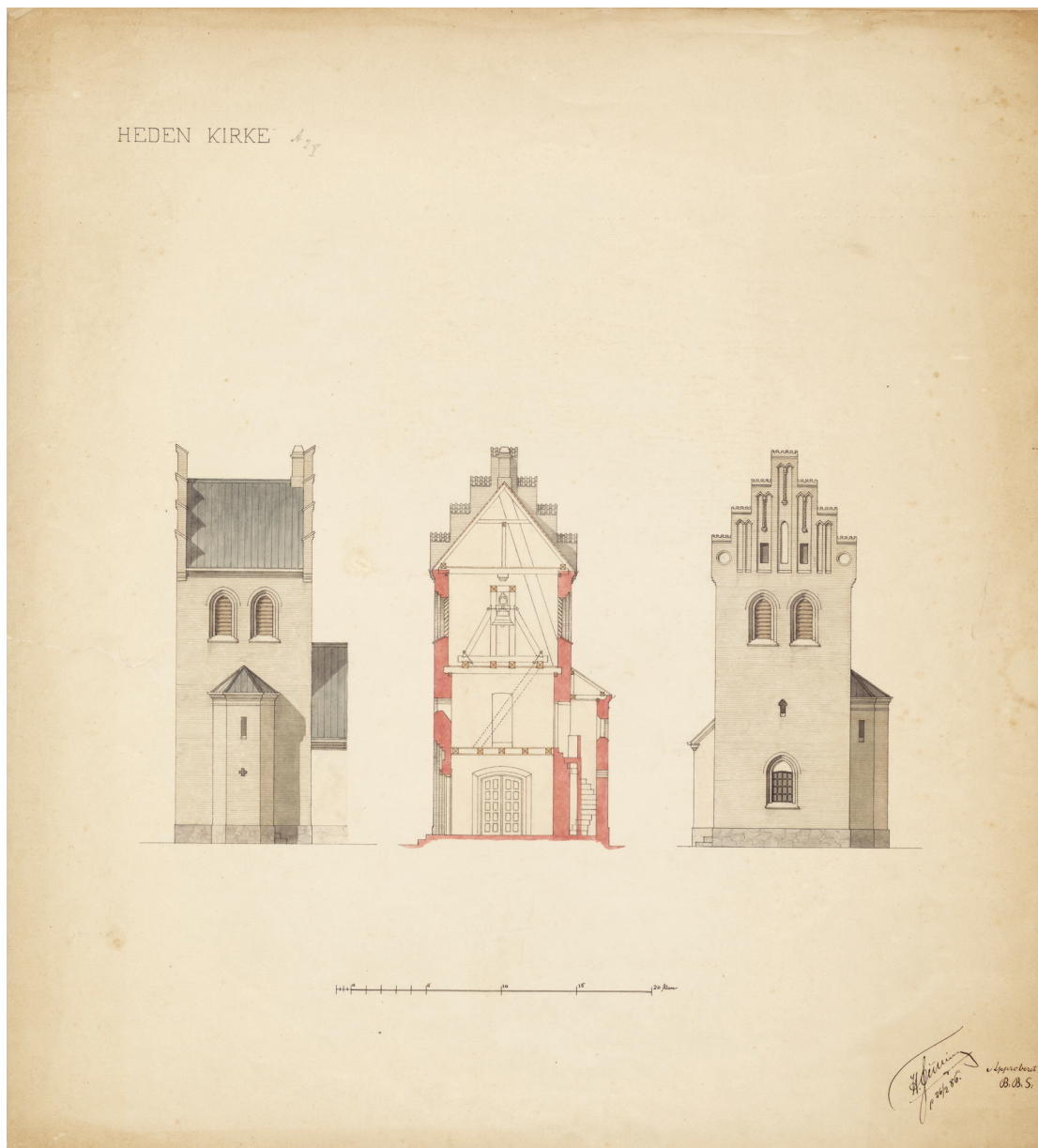
Fig. 16c-e. Tegninger til kirkens ombygning. 1:300. c. Opstalt af tårnet set fra syd. d. Tværsnit gennem tårnet set mod øst. e. Opstalt af tårnet set fra vest. Tegnet af Hans Fussing 1885-86. I Danmarks Kunstbibliotek. —Drawings for the rebuilding of the church. c. Elevation of the tower seen from the south. d. Cross-section through the tower looking east. e. Elevation of the tower seen from the west.
